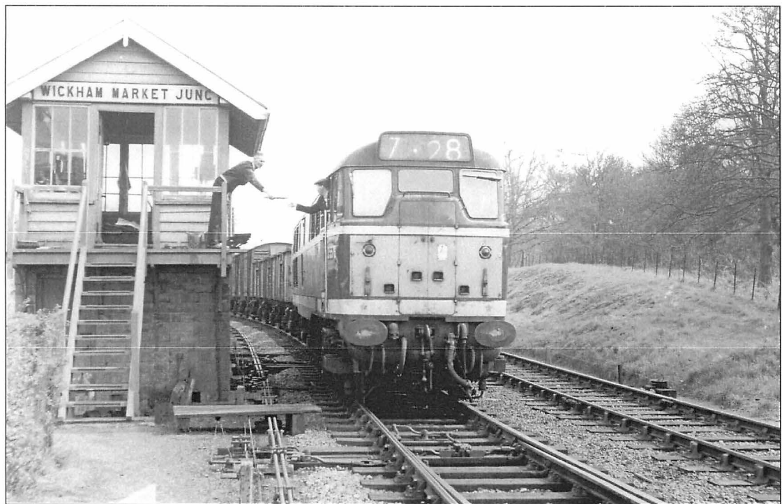
Fig. 38 Class 30 pauses in front of the points at the junction as the key is handed to the signalman. Dr. Allen.
